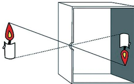
**Gambar 3.19** Kamera *Pinhole*
